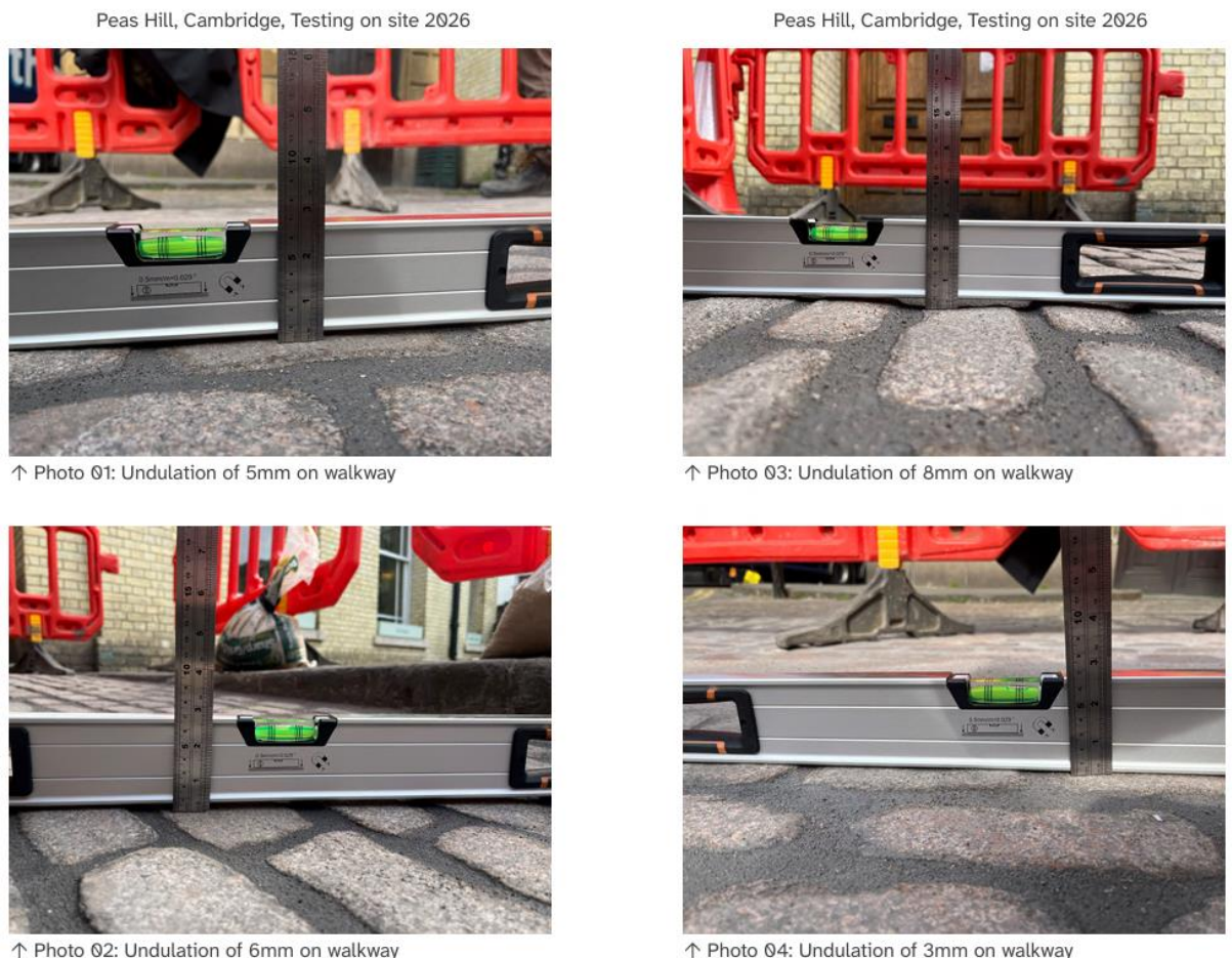
Figure 4: Photos of undulations on the trial setts, Peas Hill 2026
